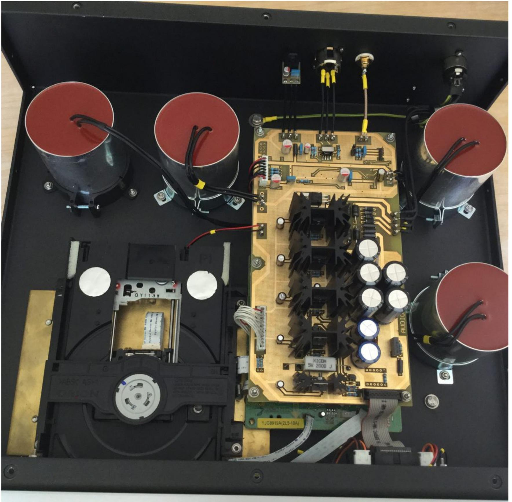
The transport drawer is treated with damping materials to reduce effects of vibration. The disc clamp mechanism features a gold plated neodymium magnet to reduce rotation related noise. The drive mechanism is coupled to a buffer circuit (2-4 seconds) for optimal resolution and low jitter. The D1 also sports blue laser diodes that bathe the read side of the CD with indirect light that supposedly improves read accuracy via a phenomenon called Stochastic resonance.
