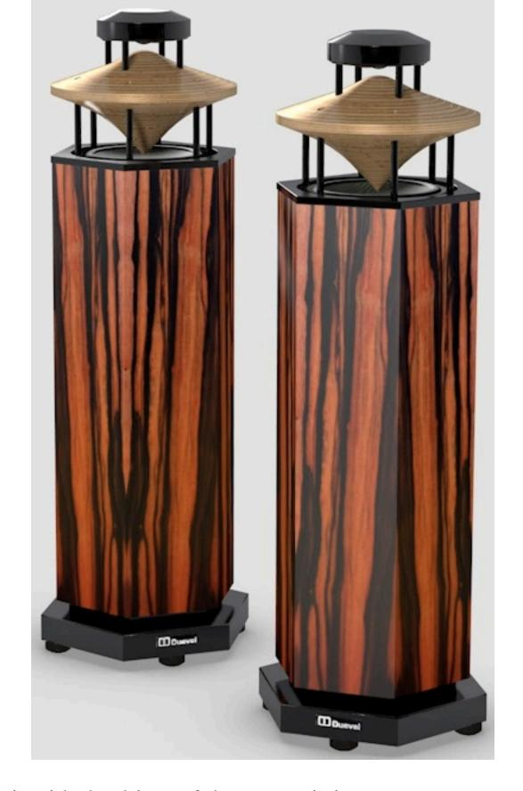
The six-sided cabinet of the Venus is just over a meter tall and is ported to the rear. An 8" carbon-fiber woofer fires up into a nicely finished wood saucer shaped radiator that disperses sound over 360 degrees. A 1" soft-dome tweeter fires down onto the top surface of the radiator. Note that the radiator is shaped differently on top and bottom to optimize the unique sound wave characteristics of both drivers.
